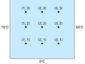
Use Liebmann's method (Gauss-Seidel) to solve for the temperature of the heated plate in figure. Employ overrelaxation with a value of 1.5 for the weighting factor and iterate to es  $\varepsilon_{\rm S}=1\%$ .
